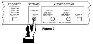
If the **LOCK** switch is engaged at any time during Test Mode, Test Mode will immediately end. The **TEST** indicator LED will be extinguished and any EVO loudspeakers will stop transmitting 'Pink Noise'.
